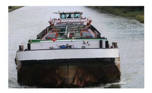
Type: motortankvessel, single hull
