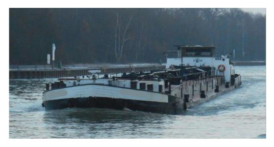
Type: Motor tank vessel, single hull
