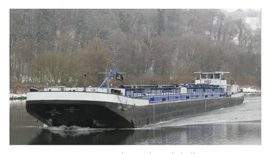
Type: Motor tank vessel, single hull
