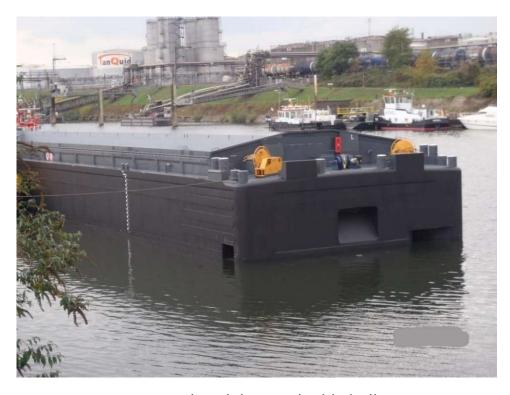
Type: steel push barge, double hull
