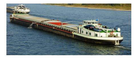
Type: dry cargo motor vessel with hatch covers
