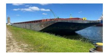
Typ: open push barge / possible with hatch covers
